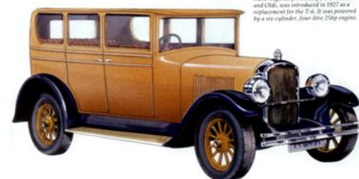
Below: The Flying Cloud, designed by John Sargent, previously from Hudson and Olds, was introduced in 1927 as a replacement for the T-4. It was powered by a six-cylinder, four-litre 21hp engine.
