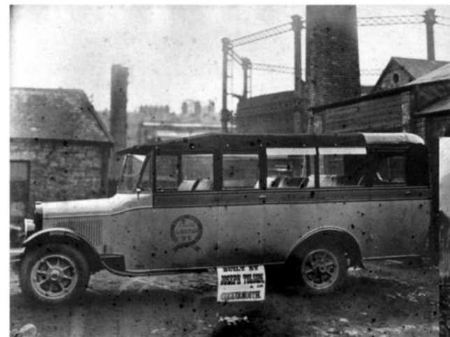
Below: The Flying Cloud, designed by John Sargent, previously from Hudson and Olds, was introduced in 1927 as a replacement for the T-4. It was powered by a six-cylinder, four-litre 21hp engine.
