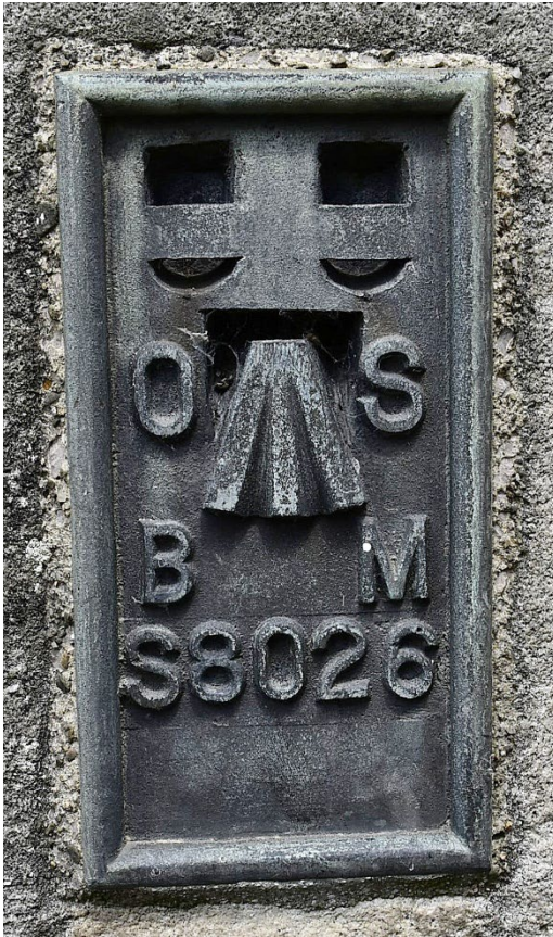
Figure 5. S-series flush bracket on wall of Bassenthwaite Lake Station House.
